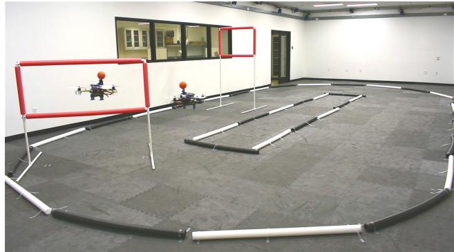
Figure 1: Drone racing experiment. Two quadrotors follow the 3-D race course while competing against the opponent quadrotor. The relative position of the opponent is detected onboard using a camera.
