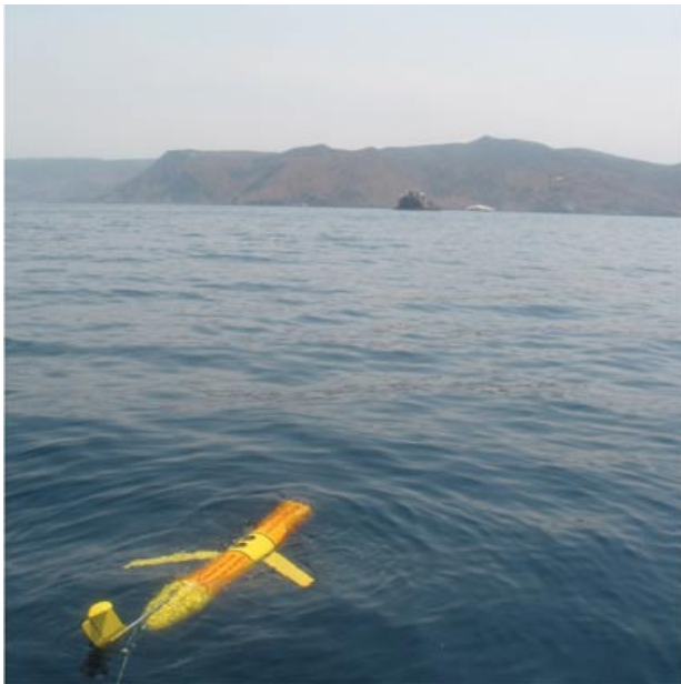
Figure 3. One of two Slocum gliders owned and operated by the USC CINAPS (Smith, Das, et al., 2010) preparing to start a mission off the northeast coast of Santa Catalina Island, California.
