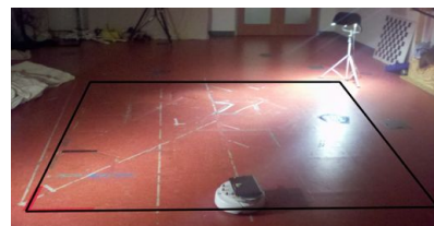
Fig. 6. The environment used in the experiments, with one robot shown. There are light sources in the bottom left and upper right corners, though the source in the lower left is not shown in the frame of the photograph. The robots' environment is the 3\text{m} \times 3\text{m} region outlined in black.
