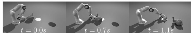
Fig. 7. We solve a push-and-slide task using trajectory optimization. The objective is to push a dynamics-augmented neural object (bunny) using a fully-actuated spherical end effector (Panda arm). The goal positions of the end effector and the bunny are shown with white and black circular targets, respectively. Leveraging the simulator’s differentiability, we optimize with a gradient-based solver a highly dynamic trajectory where the bunny slides to reach its target position.
