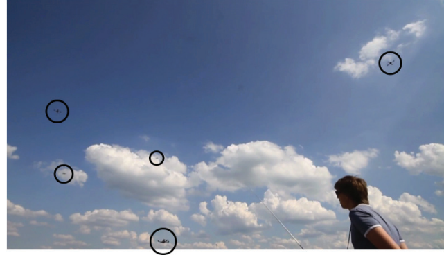
Fig. 8. This snapshot of an outdoor hardware experiment shows the autonomous deployment of five quadrotor flying robots. Even though the robots were fully autonomous, a safety pilot was assigned to each robot to allow for manual overrides in the event of an emergency.
